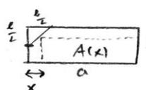
$$b \leq a \quad A(x) = (a-x) \left( \frac{b}{2} + x \right) = \frac{1}{2} ab + \left( a - \frac{b}{2} \right) x - x^2$$
