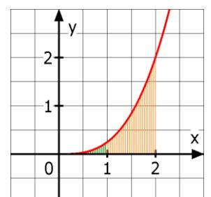
$$6. \quad A_6 = \int_1^2 0,25x^3 dx = \int_0^2 0,25x^3 dx - \int_0^1 0,25x^3 dx = 1 - \int_0^1 0,25x^3 dx$$
